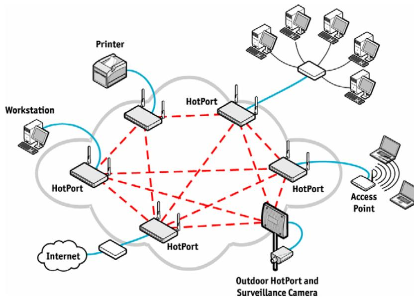
*A "mezzanine" mesh network cloud as a DMZ connected to another network*
