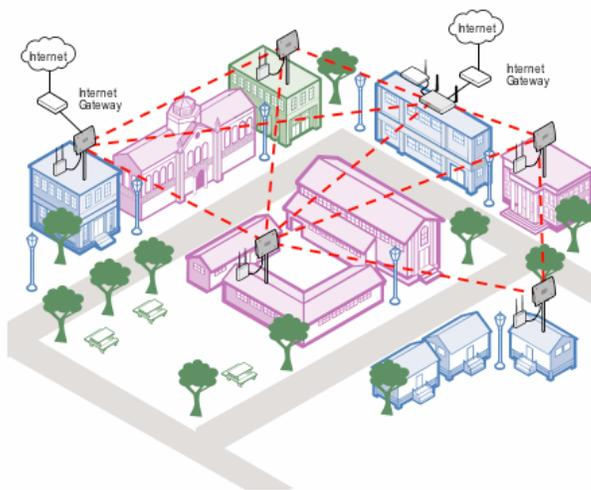
***A mesh network interfacing with access points and connecting to an enterprise/service provider network***
