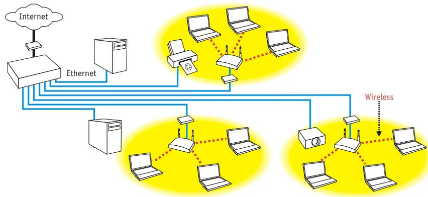
***The substantial wiring (links) required to implement a “wireless” network***
